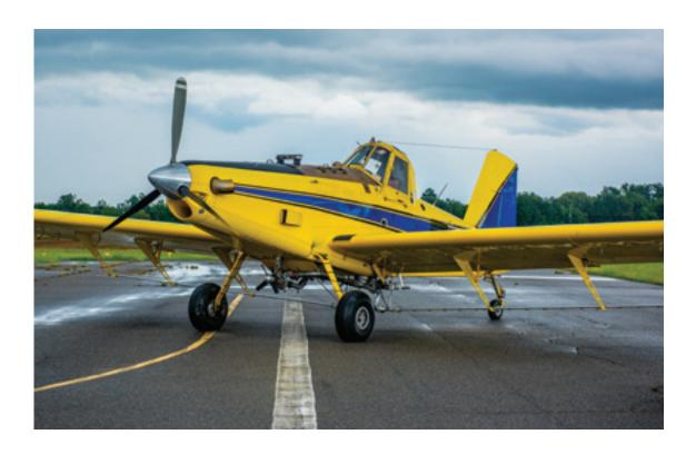
The AT-402B is designed for the operator who works off short runways or in smaller fields. With a compact, aerodynamically efficient airframe and quiet, powerful and reliable PT6A turbine engine, it is a popular choice for the operator who is moving up from smaller piston aircraft.
